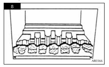
3.11 Place three large coals on the front coal so that they lean against the flame baffle, and the four large coals on the flame baffle so that they sit on the fingers, see diagram 9.
